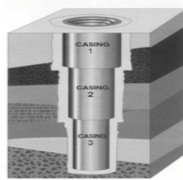
Fig. 3. Schematic [1] showing surface, intermediate and production casing phases
